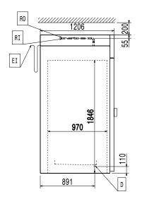
Drain Electrical inlet (power) Refrigerant Outlet
